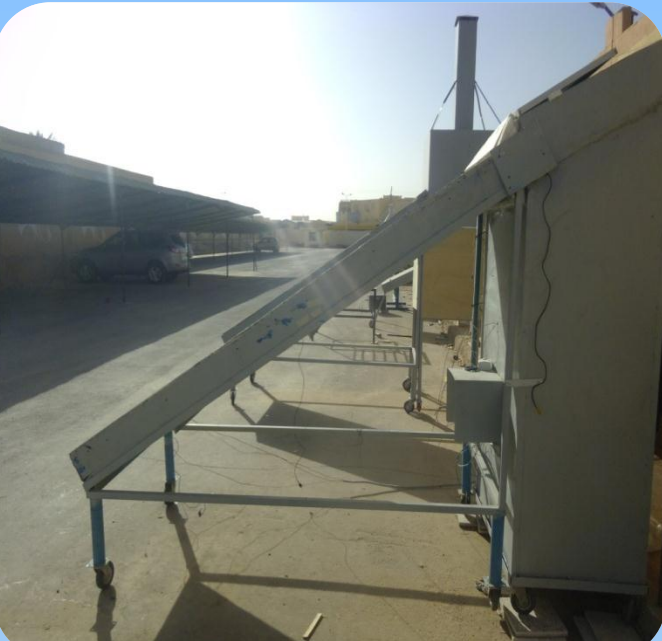
Séchoir solaire indirect a convection forcée
